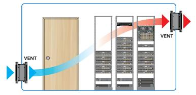
Passive cooling solution combining (2) SRCLOSETINTAKE vents, positioned to take in cool air and expel warm air.
